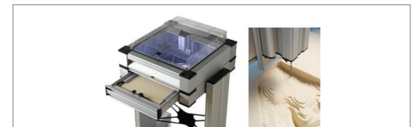
Figure 8: Desktop milling device for use in making physical compensator molds. The resolution is controlled by the size of the material subtraction bit (right panel).
